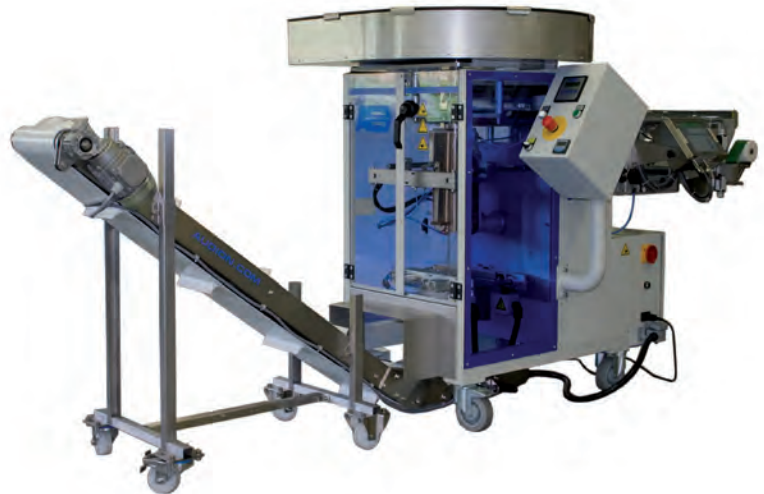
AVM 190 + sorting table, printer and conveyor
