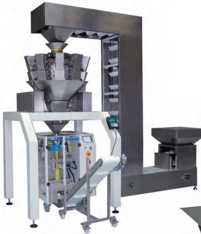
AVM 190 HS multihead scale and feeding conveyor
